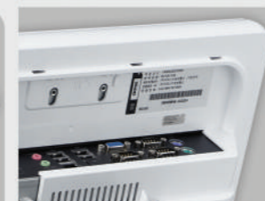
Easy to Service I/O ports are placed on the top of the panel
